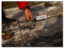
and cleaned using water (pressure wash), brushed and washed until all the limestone dust had been removed. The holes were then dried using absorbent cloth. The anchors were secured in the substrate using R-KER Epoxy Acrylate Styrene free resin. This is manufactured by RAWL Fixings. The anchors were left unloaded for 3 days until test to failure on 05<sup>th</sup> October 2011. On 05<sup>th</sup> October 2011 twelve anchors were tested to destruction.
